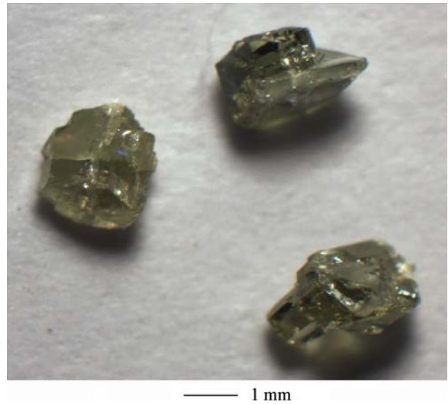
Fig. 2 \text{ZnO}_{1-x}\text{S}_x crystals ( x = 0.05 ) (diameter of the crystals up to 5 mm)
